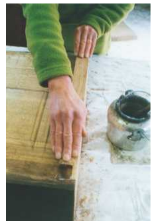
▲ Pic.1 G-clamps: the right tool for the job but keep them well padded, even on the inside of the carcass
